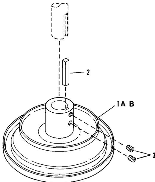
**NOTE:** Replace As Assembly Only - Special Machining Done After Hub, Pulley and Disc Assembled For These Models.
